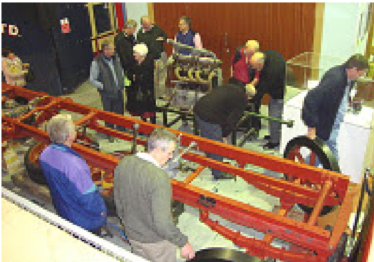
Chassis: the trial build of the freshly primed frame and brackets.
